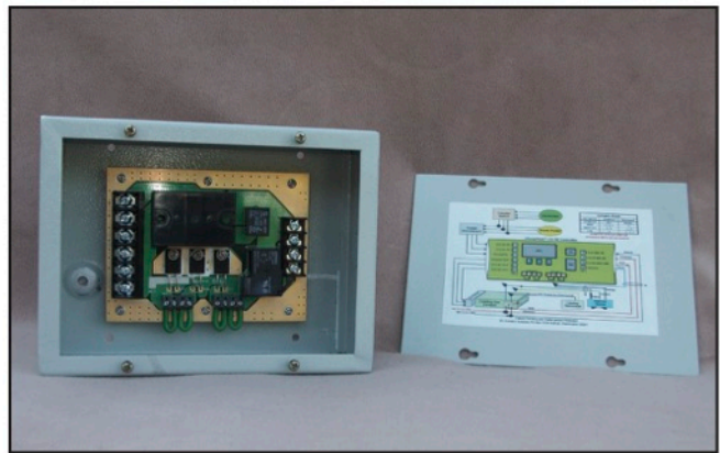
The CheapHeat System is comprised of a few key components, including the controller box (pictured). The controller ties the CheapHeat system together with the existing wall thermostat and fan.
